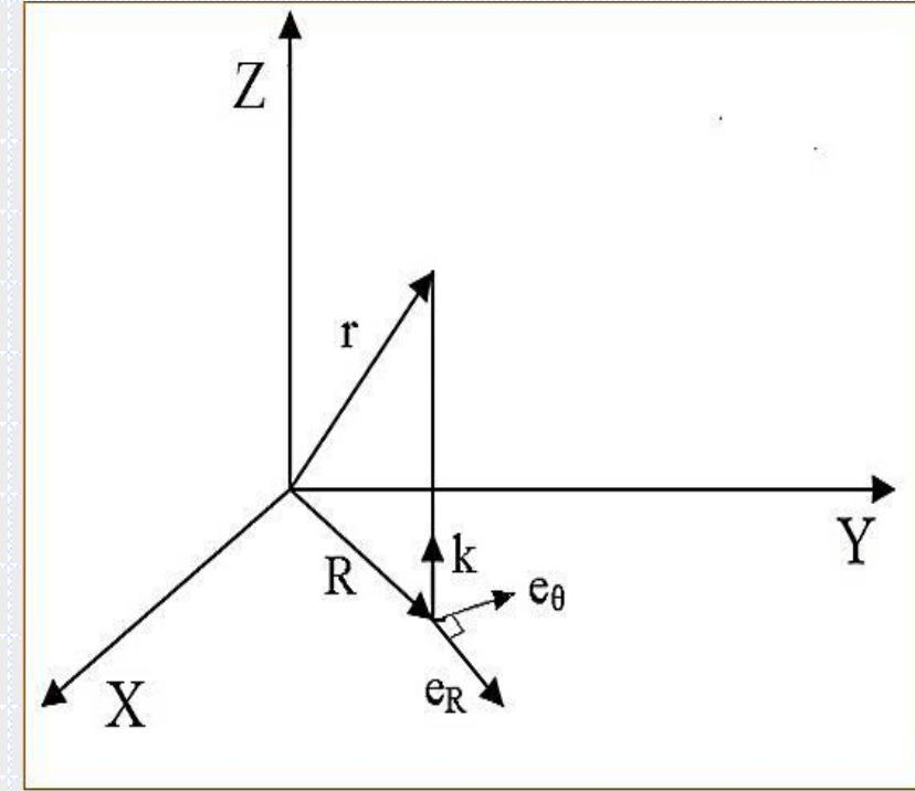
$$v_R = \dot{R}, \quad v_\theta = R \dot{\theta}, \quad v_z = \dot{z}$$
