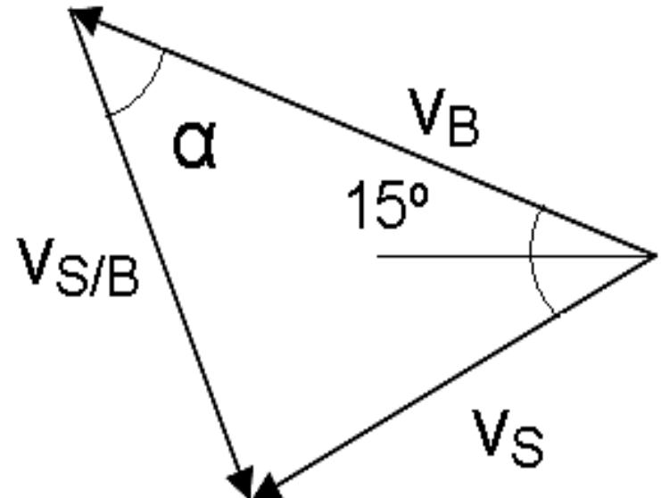
$$v_{S/B} = \sqrt{v_B^2 + v_S^2 - 2v_B v_S \cos(86.5)} = 20.01 \text{ ft/s}$$
