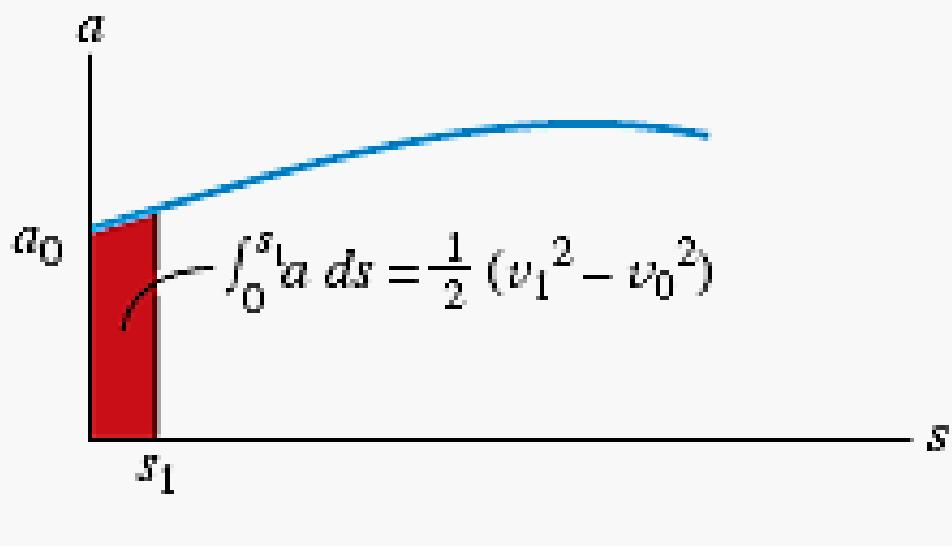
$$\int_{s_0}^{s_1} a \, ds = \frac{1}{2} (v_1^2 - v_0^2)$$
