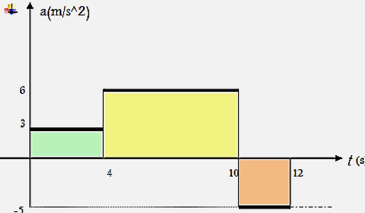
$$a = \frac{dv}{dt} \Rightarrow dv = a dt \Rightarrow \int_{v_0}^{v_4} dv = \int a dt = \int_0^t a dt$$
