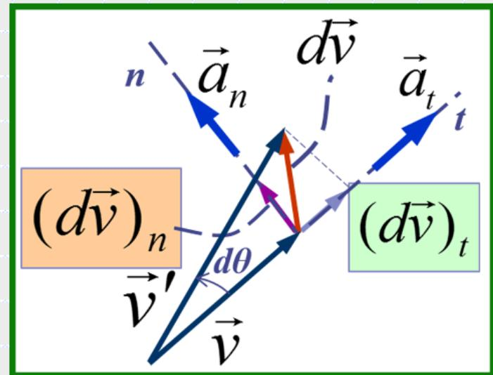
$$\begin{aligned} d\vec{v} &\approx (d\vec{v})_t + (d\vec{v})_n \\ &\approx |(d\vec{v})_t| \hat{e}_t + |(d\vec{v})_n| \hat{e}_n \end{aligned}$$
