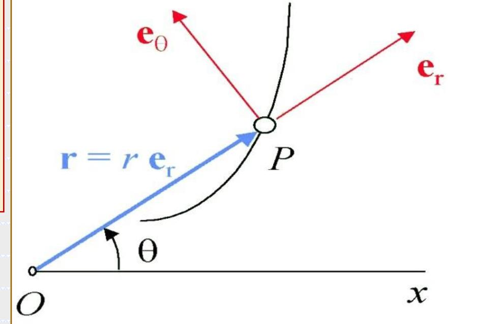
$$\vec{r} = r \vec{e}_r \quad \Rightarrow \quad \vec{v} = \frac{d\vec{r}}{dt} = \frac{d(r\vec{e}_r)}{dt} = \frac{dr}{dt} \vec{e}_r + r \frac{d\vec{e}_r}{dt}$$
